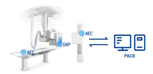
The AEC (Automatic Exposure Control) function controls the X-ray dosage to prevent the patient from being exposed to unnecessary radiation. The DAP sensor of the collimator shows the X-ray dosage for the patient and the operator can manage the dosage effectively by utilizing the DAP information sent to the PACS.
